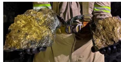
Initial sampling at PC Shaft revealed grades in excess of 300g/t, containing large amounts of visible gold
